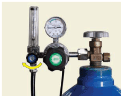
Control flow rate by turning pressure control lever. (Based on \varnothing 0.8 mm)
