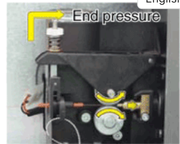
Connect new wire to feeder and switch on the welding torch to discharge wire
