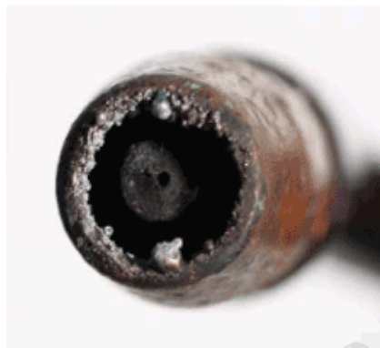
Adherence of spatter onto nozzle and contact tip after welding
