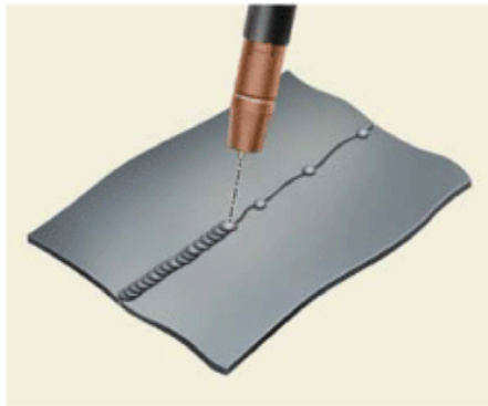
Forced continuous welding can result in excessive thermal deformation.
