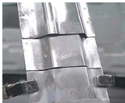
Opening for filler and reinforcement panel is the same as panel thickness.
