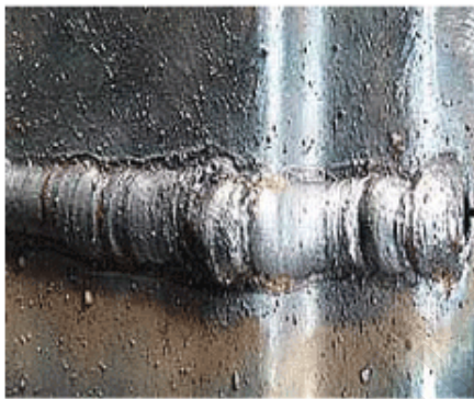
Defective welder voltage and torch speed
