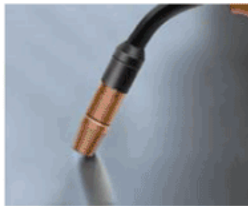
Remove twisted wire and discharge wire inside welding torch
