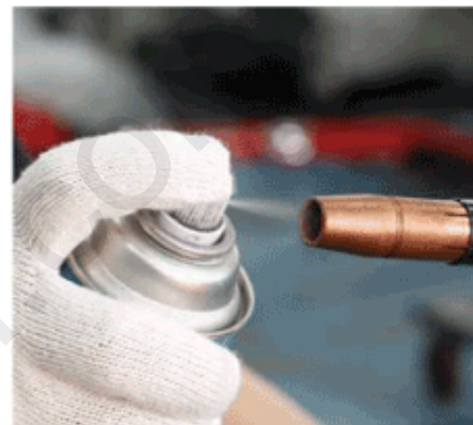
Weld after applying anti-spatter compound
